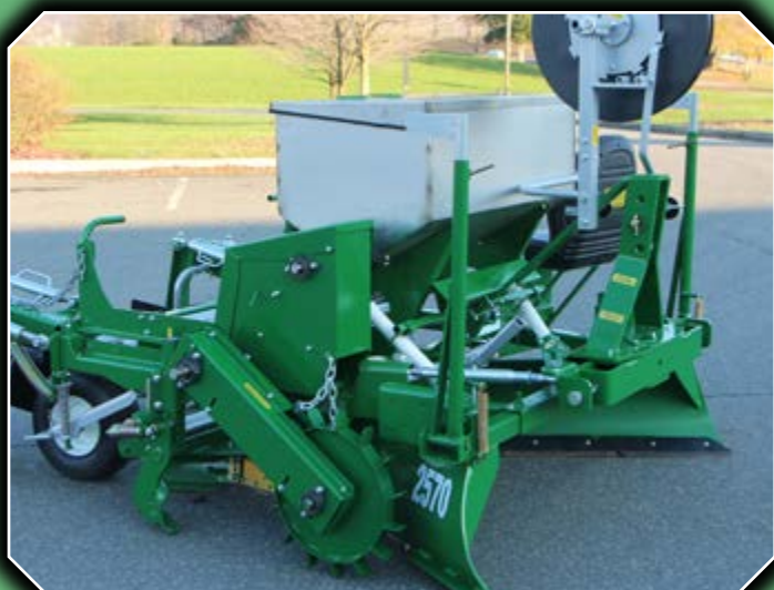
Drive Wheel and Gear Box
