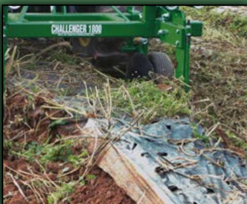
Automatic Reset Without Center Coulter
