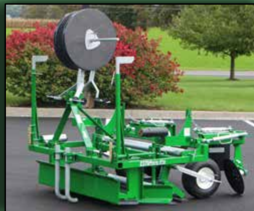
Trench Opener & Leveling Blade
