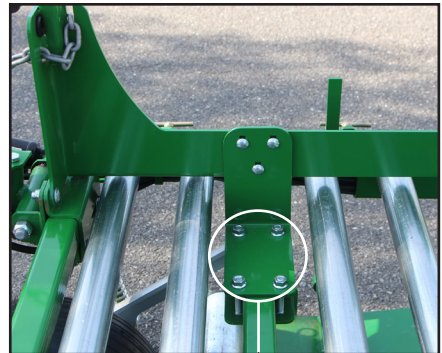
(No.4) Roll holder and tire adjustment
