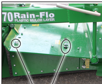
(No.3) Remove bolts from bed press side plates and move to appropriate setting. NOTE; For straight beds, each side must be equally adjusted.
