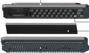
Extra Large Flow Labyrinth reduces pressure while forming high turbulence in the dripper to keep solids in suspension. Most plug resistant flow path in the industry.
